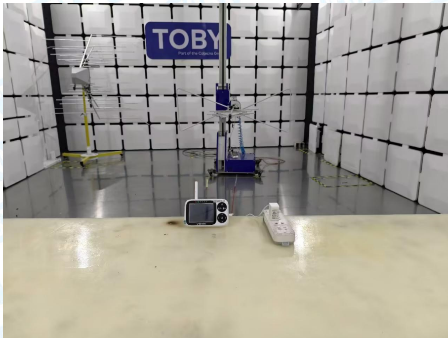
Photo of Setup for Radiated Emission (30MHz~1GHz)
