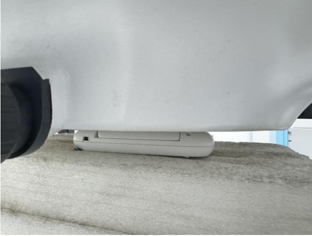
Body worn –Back-antenna folded (0mm)
