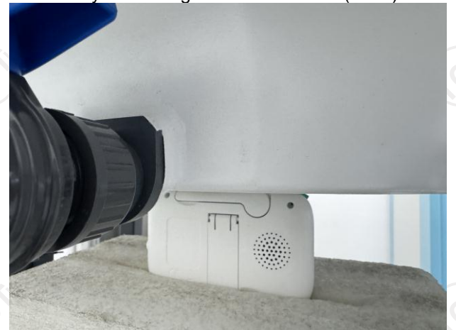
Body worn –Top-antenna folded (0mm)
