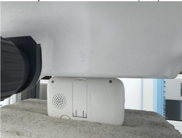
Body worn –Bottom-antenna folded (0mm)
