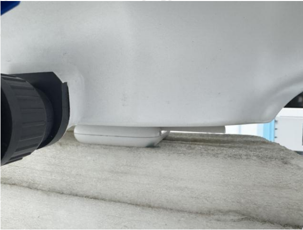
Body worn –Back-antenna unfolded (0mm)
