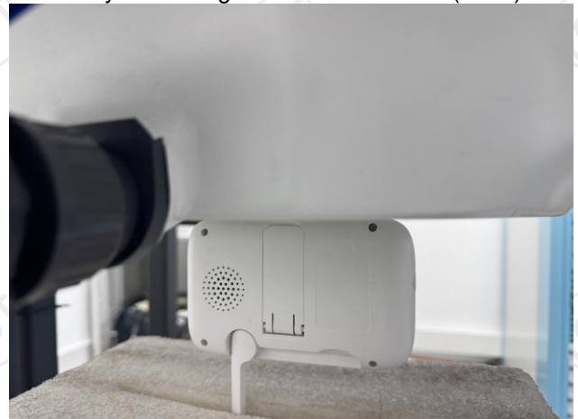
Body worn –Bottom- antenna unfolded (0mm)
