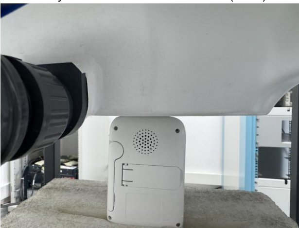
Body worn –Left-antenna folded (0mm)
