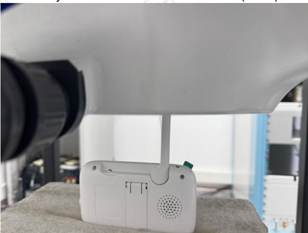
Body worn –Top- antenna unfolded (0mm)
