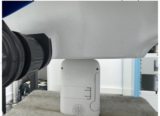
Body worn –Right-antenna folded (0mm)
