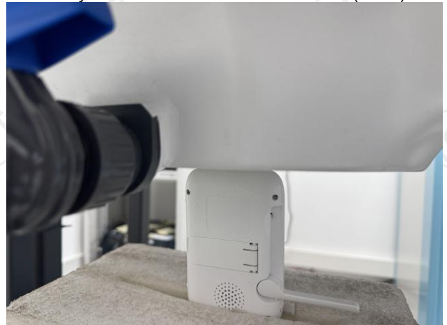
Body worn –Right-antenna unfolded (0mm)
