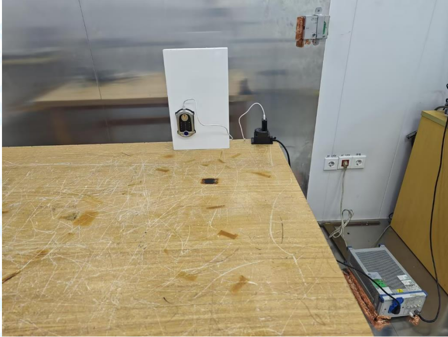
Photo of Setup for Radiated Emission (0.009MHz-30MHz)
