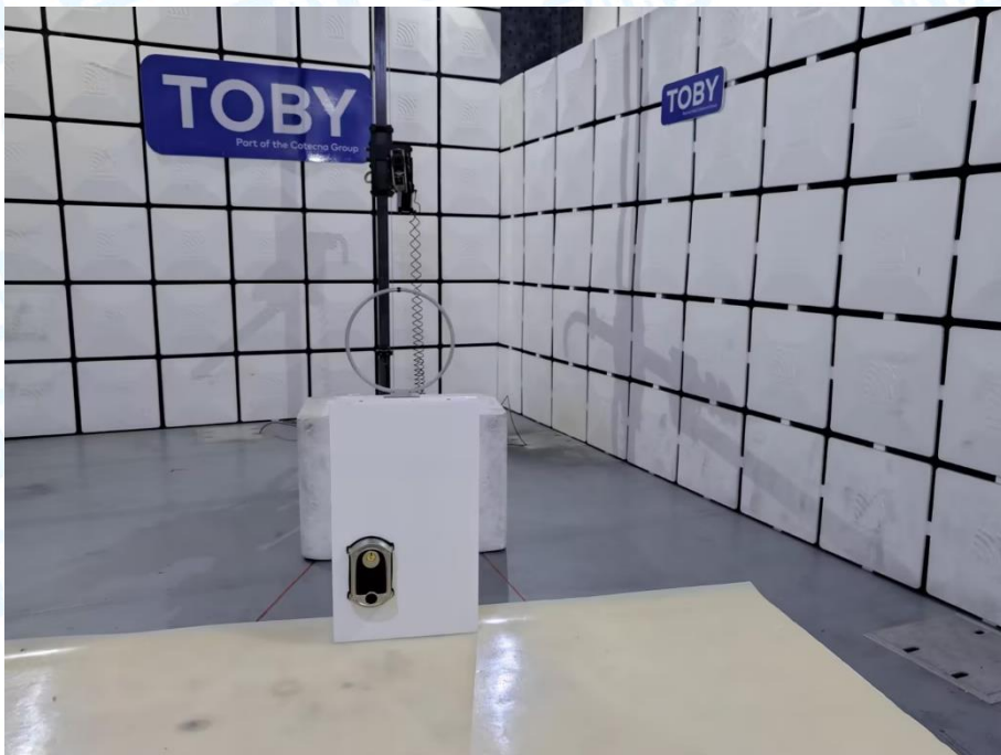
Photo of Setup for Radiated Emission (0.009MHz-30MHz)
