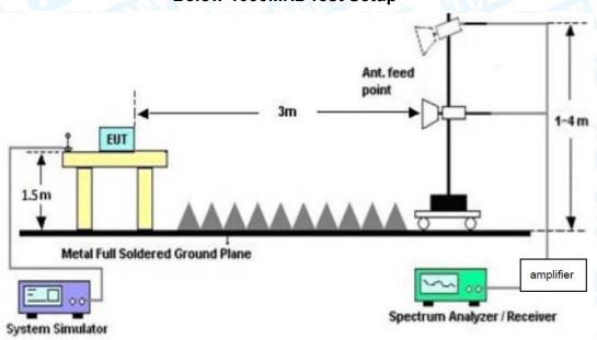
**Above 1GHz Test Setup**
