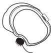
2. Woolen horn Velcro installation At the location of the ear protectors on both sides Install the headphones
