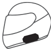
5. Mao Mian Host Velcro Installation In a suitable position on the left side
