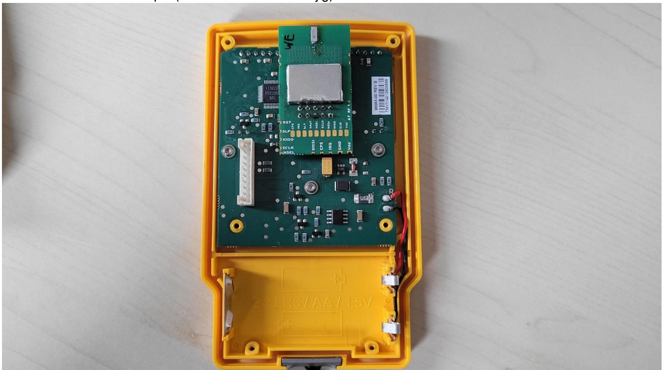
Photo No. 4: radiated sample (module installed in test jig)
