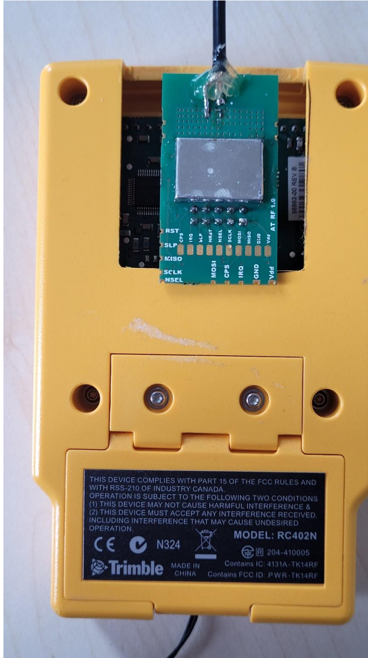
Photo No. 6: conducted sample (module installed in test jig)
