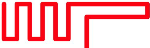
A red line drawing of a meander line antenna, consisting of a series of zig-zag turns followed by a straight vertical segment on the right.
