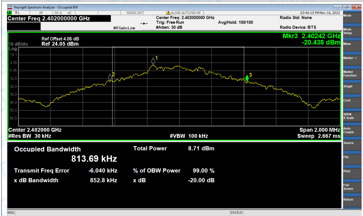
-20dB Bandwidth NVNT 1-DH1 2441MHz Ant1
