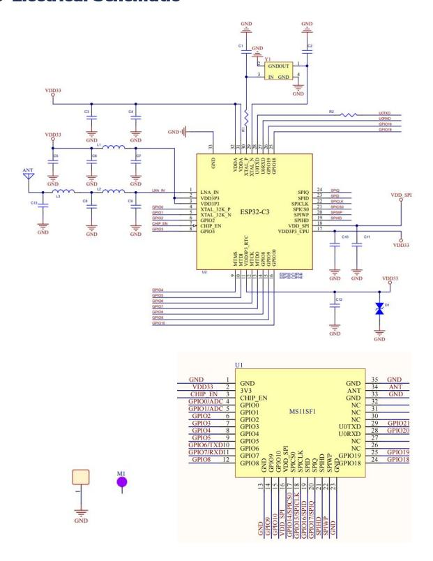
**Notice:** If you need to use an external antenna annoying please contact the salesman, need to internally modify the  $0 \Omega$  resistor connection direction.
