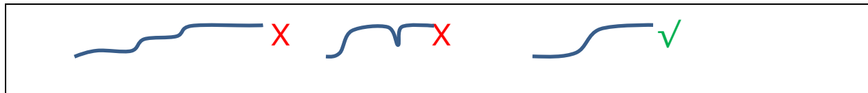
Figure 3-1 Power supply rise flow
