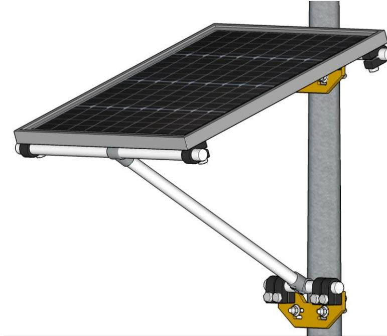
**Fig 6: Solar panel on a utility pole**
