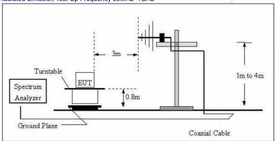
(C) Radiated Emission Test-Up Frequency Above 1GHz
