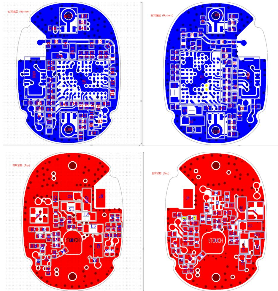
Link by Eargo is wireless Bluetooth TWS earbuds, a pair of earbuds are divided into left and right earbuds, the appearance is different, but the internal PCBA circuits are identical. It's because the earbud structure is mirrored, resulting in PCBA appearance differences.
