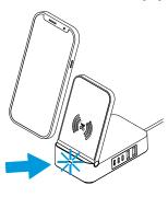
Blue solid light means the device is charging.
