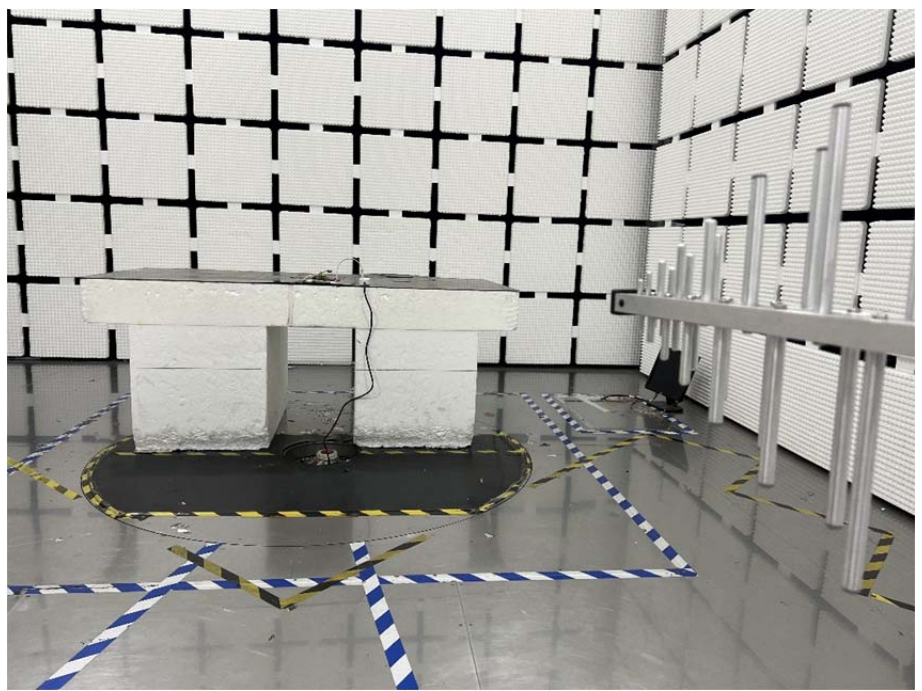
Radiation Emission Test Setup (30MHz to 1GHz)
