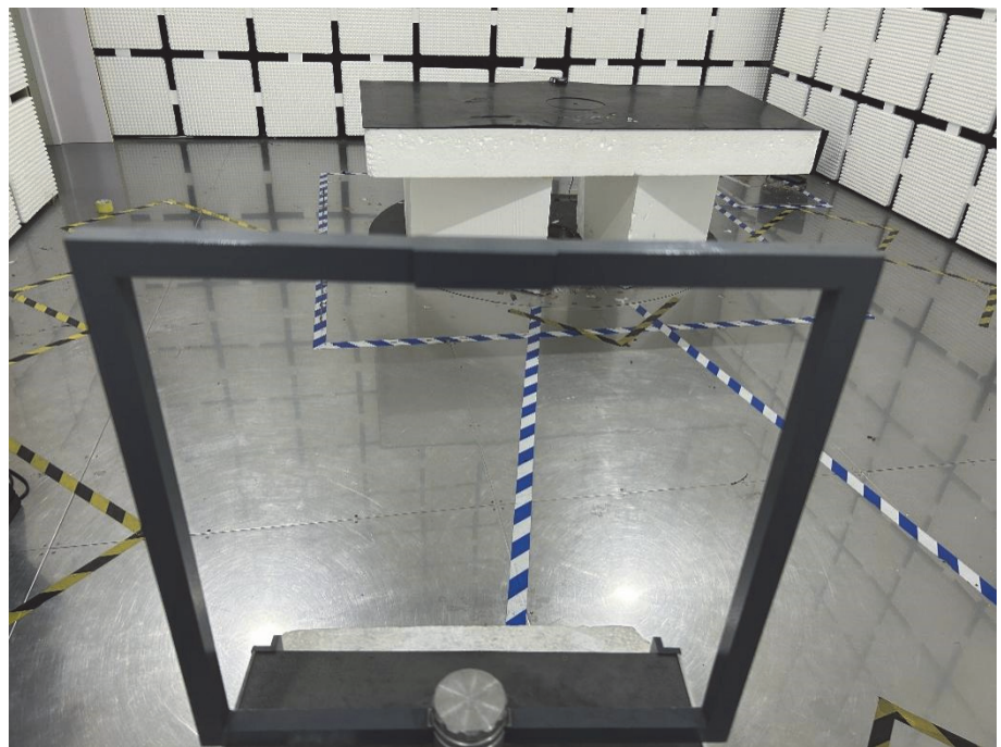
Radiation Emission Test Setup (Below 30MHz)
