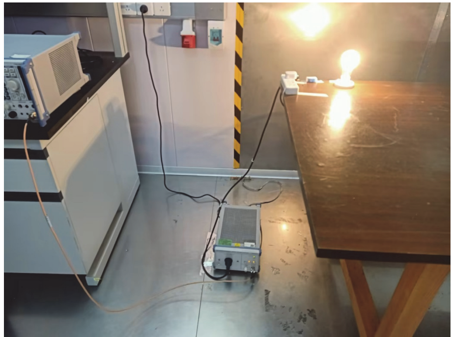
Conducted Emission Test Setup
