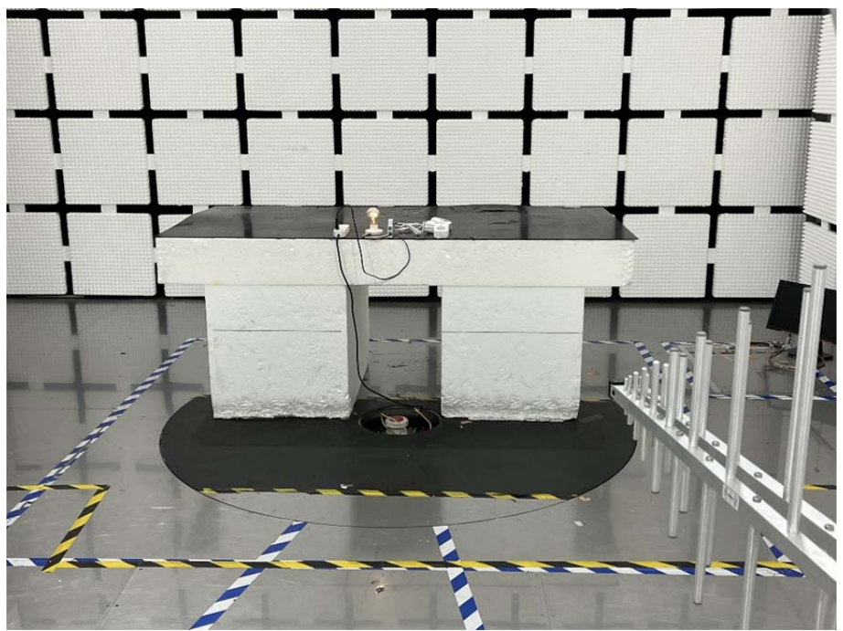
Radiation Emission Test Setup (30MHz to 1GHz)
