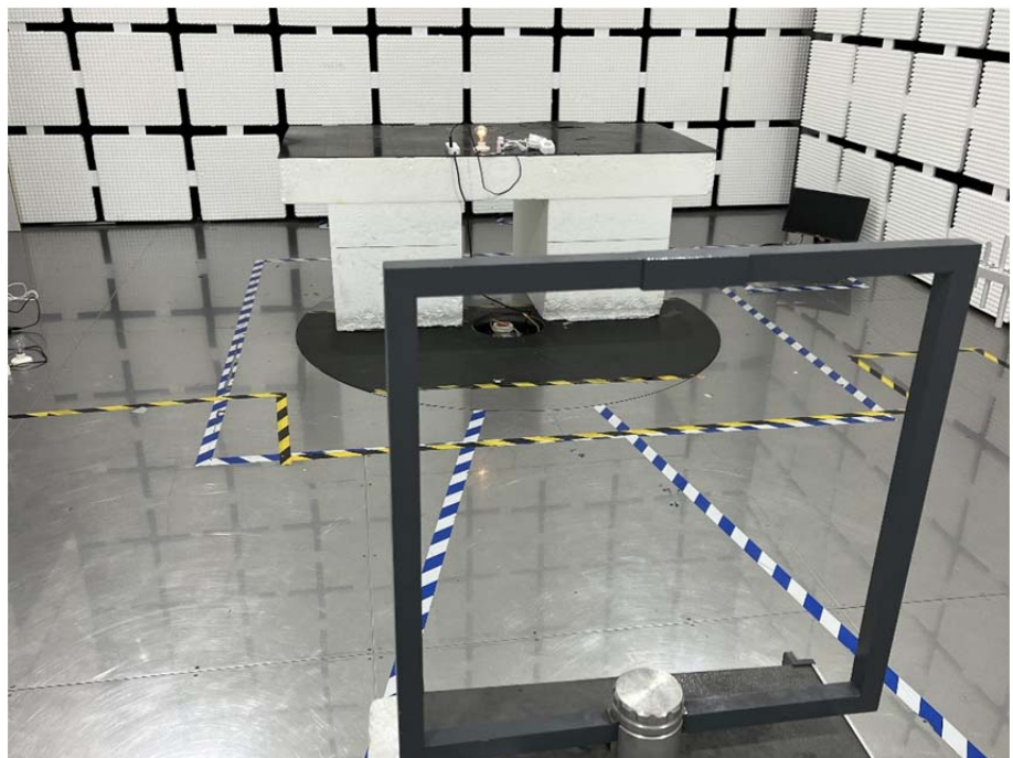
Radiation Emission Test Setup (Below 30MHz)
