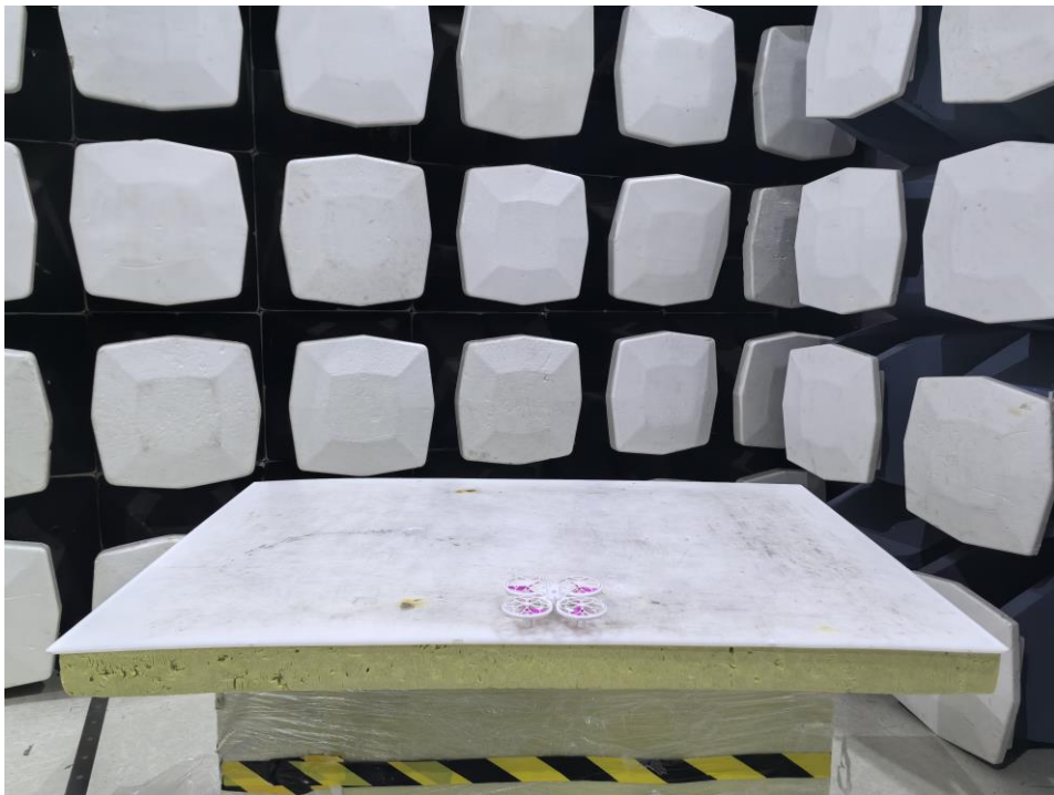
Up to 1GHz (EUT was placed in the centre of the turntable)
