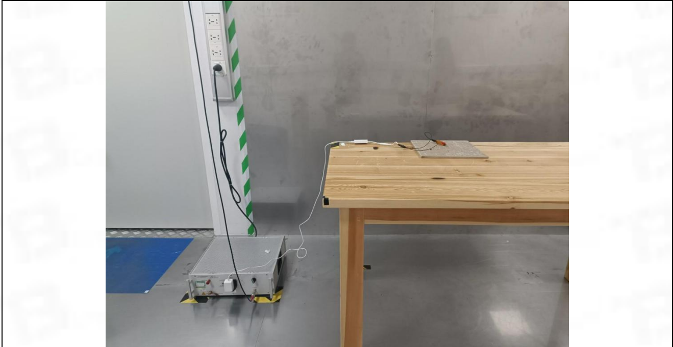
Conducted Emission at AC power line
