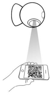
At the same time, keep an eye on the **flashing blue** LED on the camera, when it becomes **Steady Blue**, the scan is successfully. You can stop letting camera scanning the code and just wait for several seconds.
