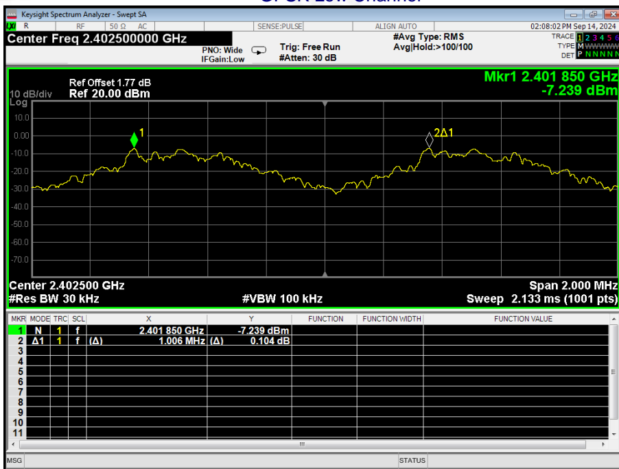
Test plots GFSK Low Channel
