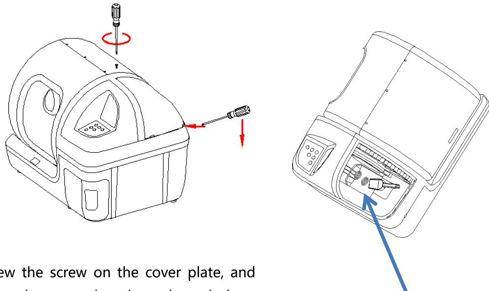
Unscrew the screw on the cover plate, and then pry the cover plate down through three gaps with a screwdriver.
