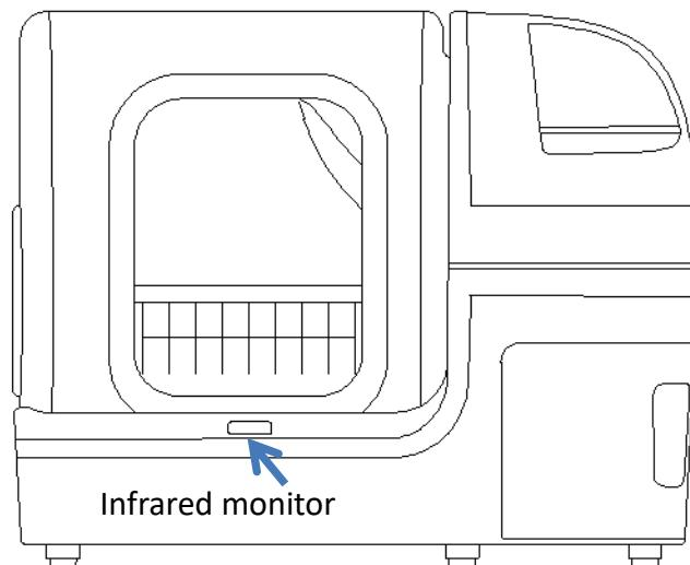
Please keep the infrared monitor panel clean during use to avoid monitoring errors
