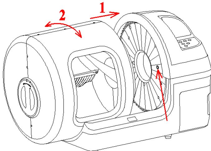
Align the circular silicone marks on the drum and on the gear. Follow the arrow 1 and then arrow 2 direction until the drum is secured.
