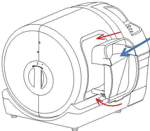
2, Install the cat litter clearing frame on the entrance/exit according to the arrow direction. Note: it must be buckled in place
