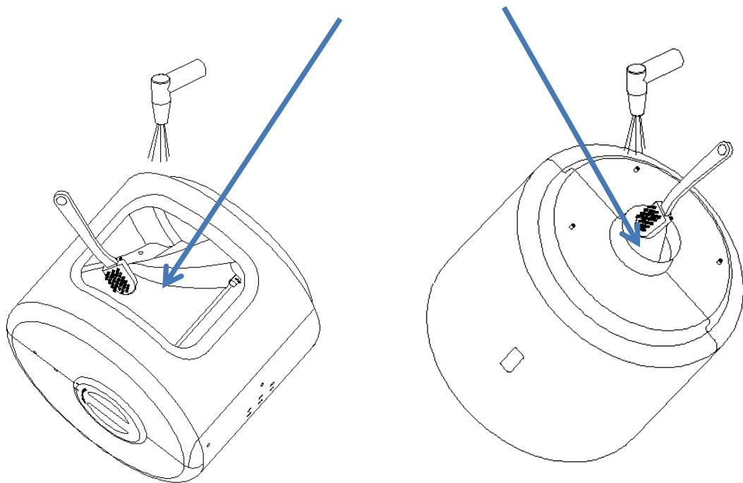
**Note: After washing the drum, place it in a ventilated place and dry it thoroughly before using it again.**
