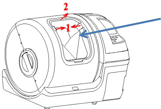
4, Remove the cat litter clearing frame as shown in the arrow and keep it properly.
