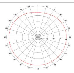
Far-field Power Distribution(H+V) on X-Y Plane Plot Peak Gain(H+V)= -0.70 dBi; Plot AvgGain(H+V)=-2.73dBi @2450 MHz
