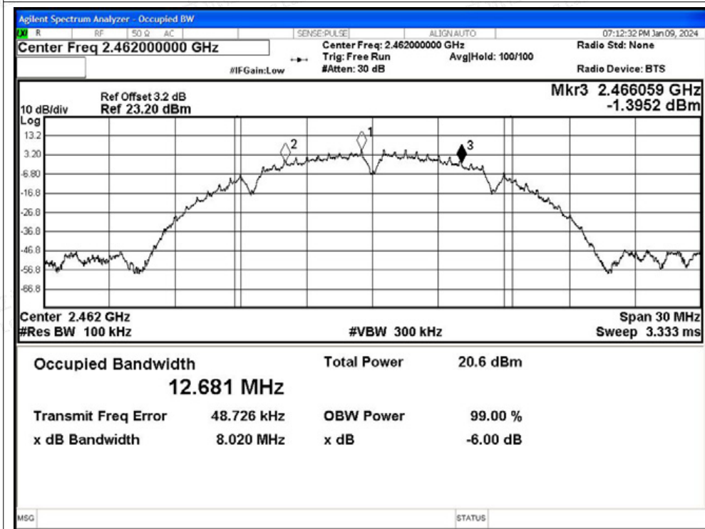
-6dB Bandwidth NVNT g 2412MHz Ant1
