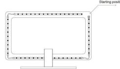
1.When the strip light is slightly longer than the edges of the TV, you can bend and paste the light strip.
