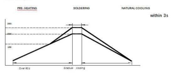
Recommended temperature profiles for re-flow soldering in Figure 1.
