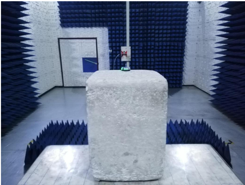
RADIATED EMISSION TEST SETUP ABOVE 1GHz
