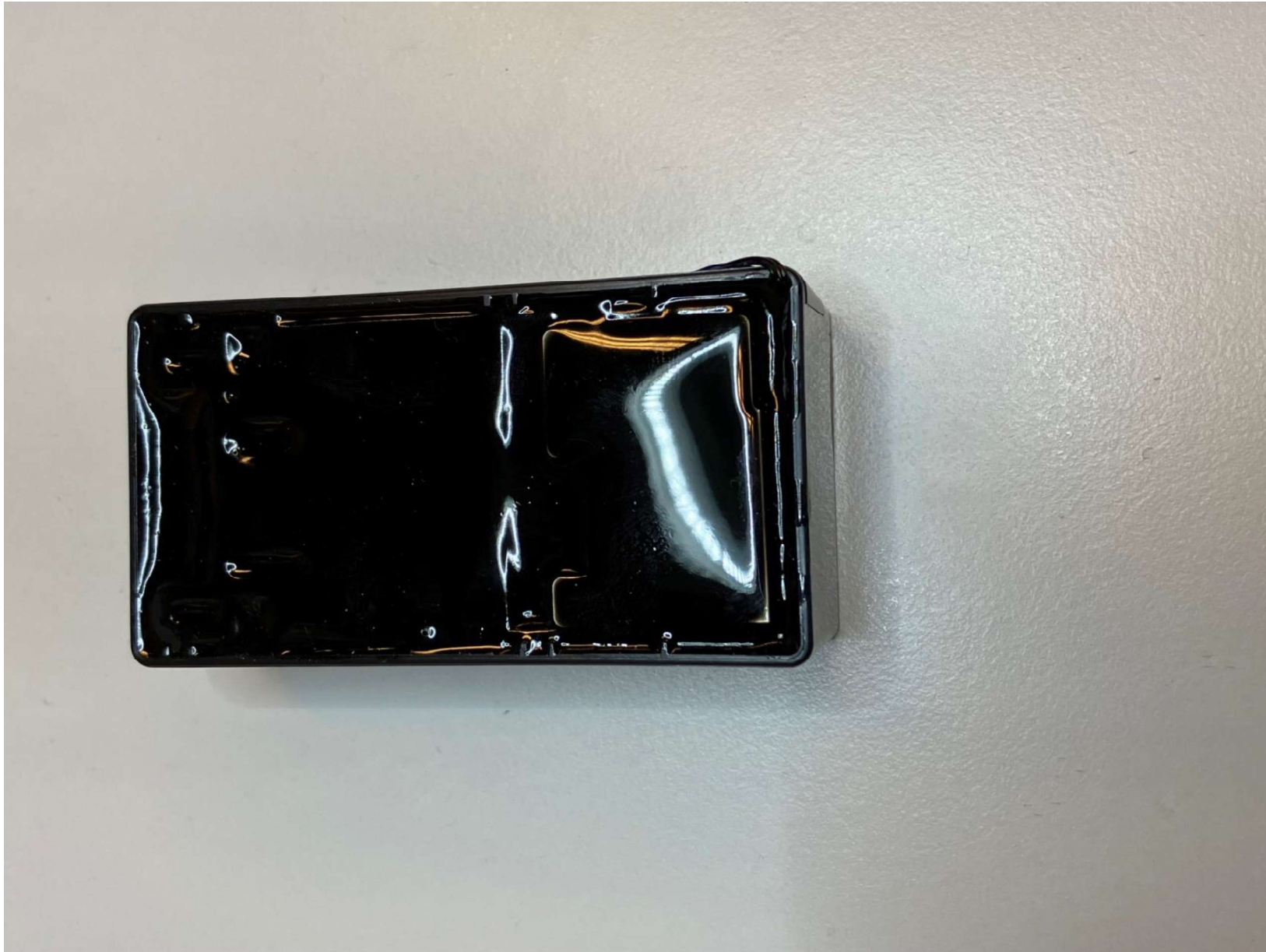
Power pack assembly with main PCB inside inner box filled with potting material
