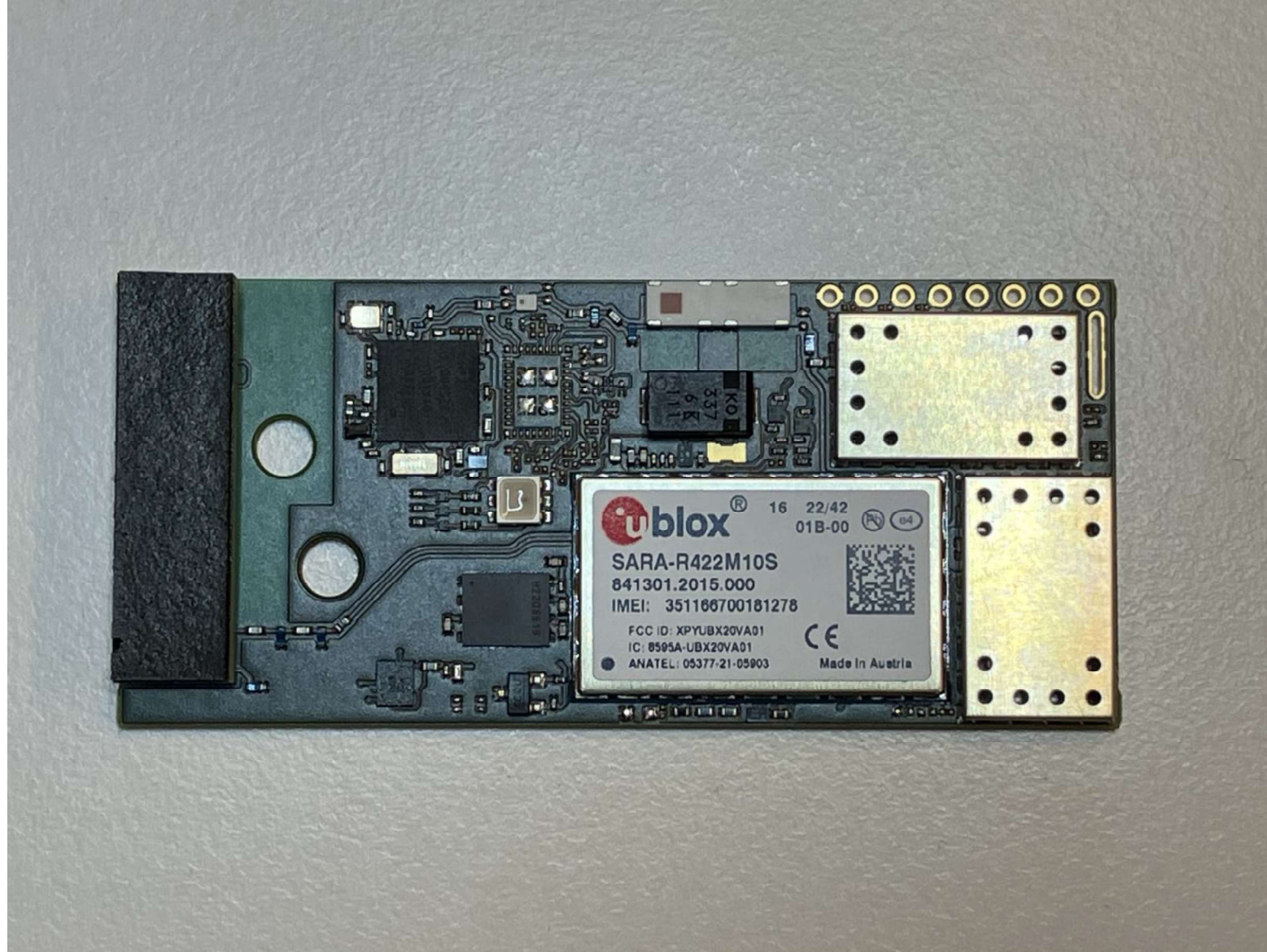
Main PCB top with shields and antenna gasket
