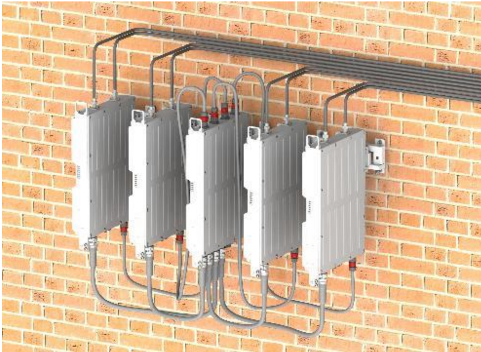
Figure 4-32 Connection for RF cables between MCU and LPAs
