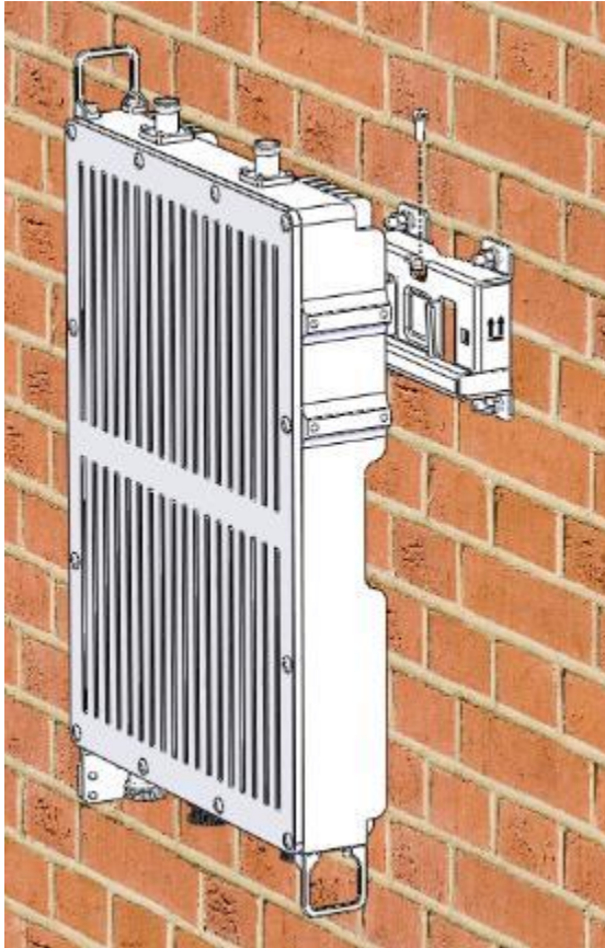
Figure 4-23 Put the device on the support and tighten the screws
