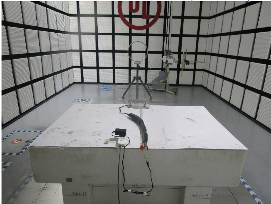
RADIATED RF MEASUREMENT SETUP (Below 30MHz)
