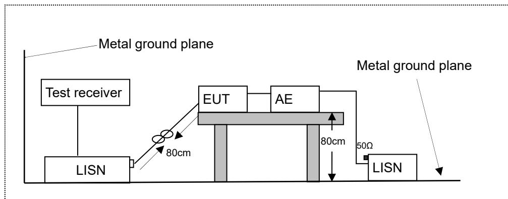
LISN: Line Impedance Stabilization Network
