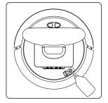
4.①Open the flip panel ②Turn on the water filling plug ③Use the special bottle to add water(less than100ml) It is strictly prohibited to use other bottles for water injection
