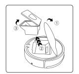
7.①Open the magnetic cover,②Raise upward the dust box,③Open the dust box to take out the garbage and reload the box
