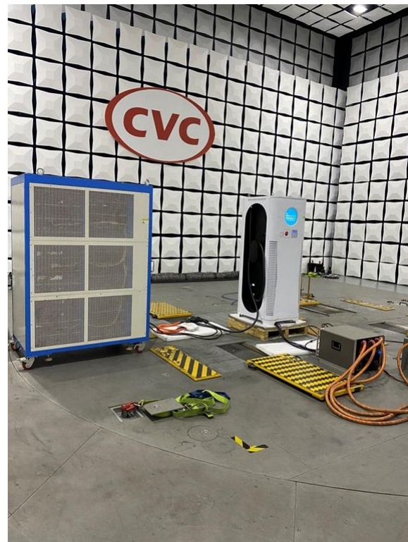
Setup photo of conducted emission (150KHz-30MHz)
