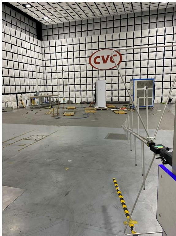
Setup photo of radiated emission (30MHz-1GHz)
