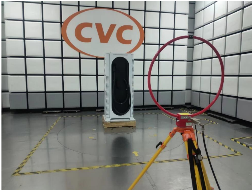
Setup photo of radiated emission (9KHz-30MHz)
