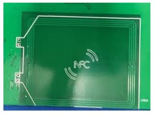
Antenna transmission frequency: 13.56 MHz Antenna type: PCB antenna
