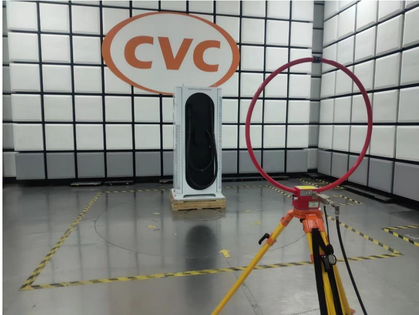
Setup photo of radiated emission (9KHz-30MHz)
