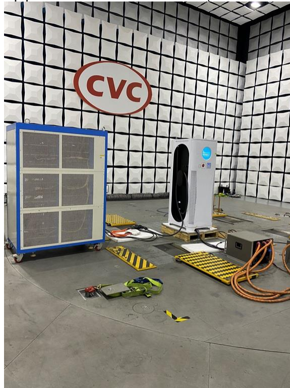
Setup photo of conducted emission (150KHz-30MHz)
