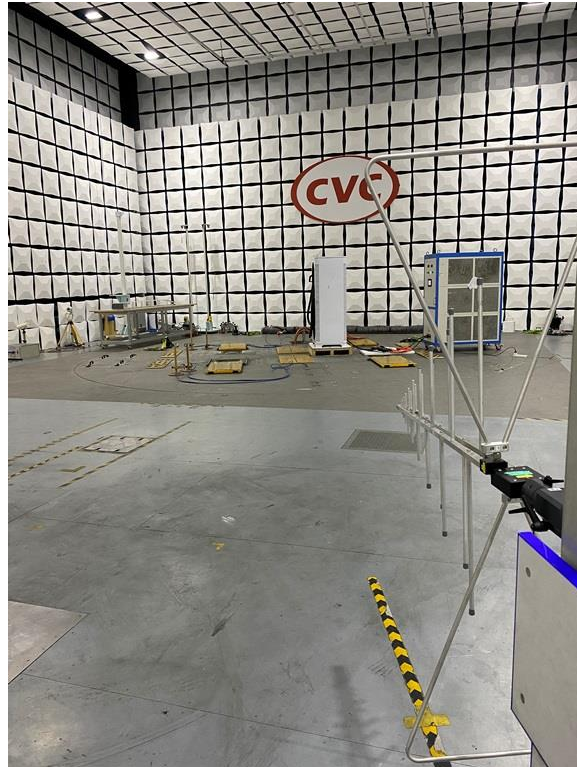
Setup photo of radiated emission (30MHz-1GHz)
