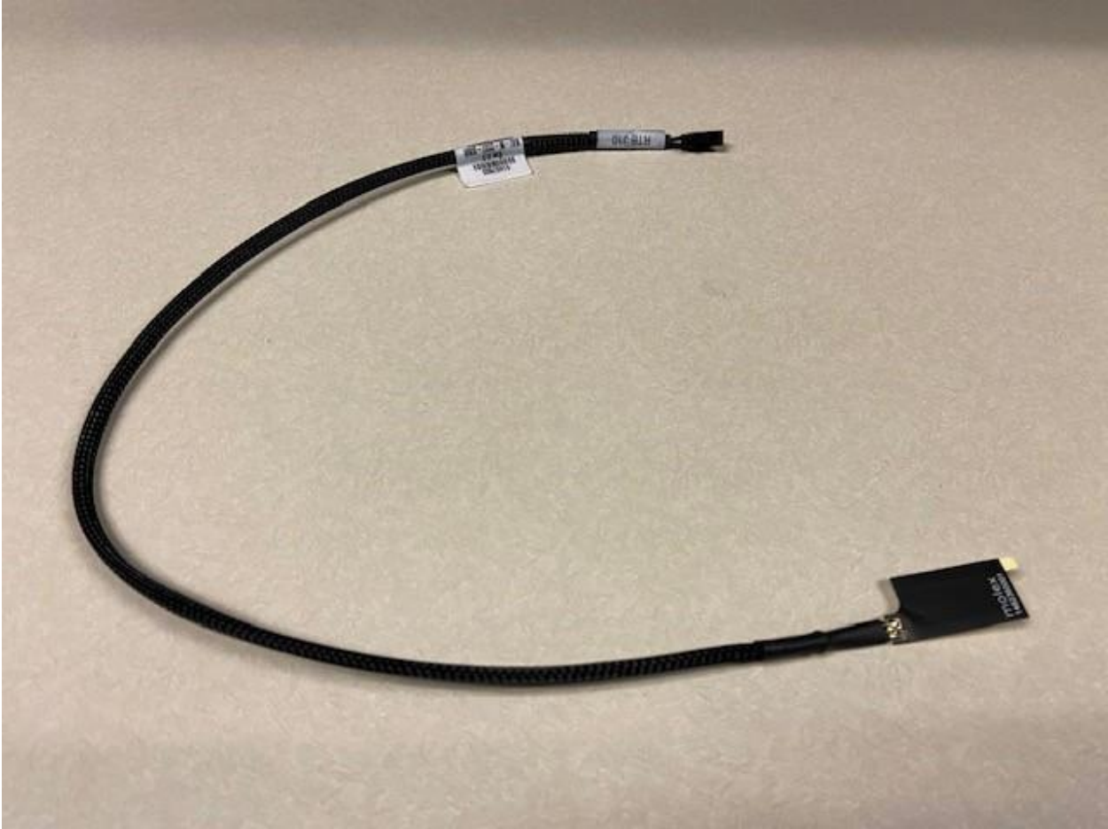
Figure 6: NFC Antenna harness prior to assembly in console.
