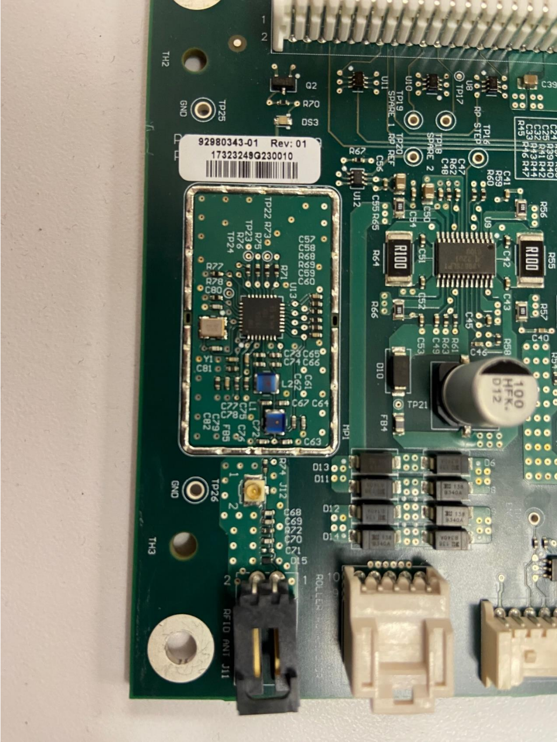
Figure 2: Roller Pump PCA – close up of radio circuitry.
