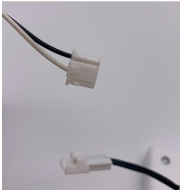
Installation is as easy as connecting this cable, then mounting the communication card to the piece of equipment using the hook feature on the rear of the device. Some devices like the automated flush valve below need to be partially disassembled to allow the hook feature to be “captured” by the equipment’s metal or plastic enclosure. Once mounted, the assembly should appear similar to the below image.
