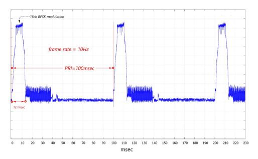
Duty cycle correction = 10log(Ton/T) On time = 13.1 \* 3 = 39.3 ms 39.3/230 = 0.17087 10\*Log (0.17087) = 7.67dB
