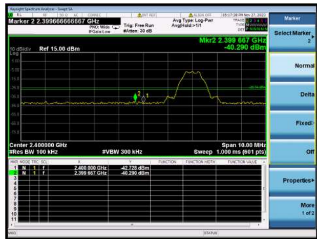
GFSK (BLE 1Mbps) HIGH CHANNEL, BAND EDGE
