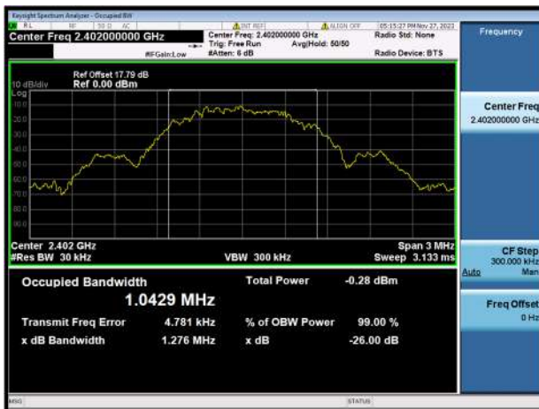
GFSK (BLE 1Mbps) LOW CHANNEL
