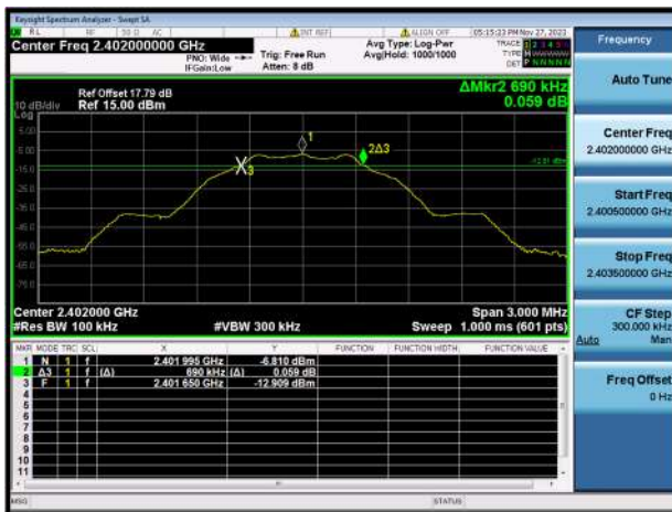
GFSK (BLE 1Mbps) LOW CHANNEL
