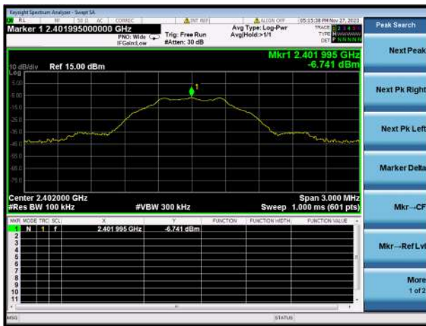
GFSK (BLE 1Mbps) LOW CHANNEL, CARRIER LEVEL
