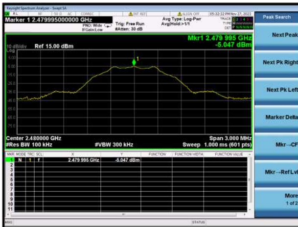
GFSK (BLE 1Mbps) HIGH CHANNEL, CARRIER LEVEL
