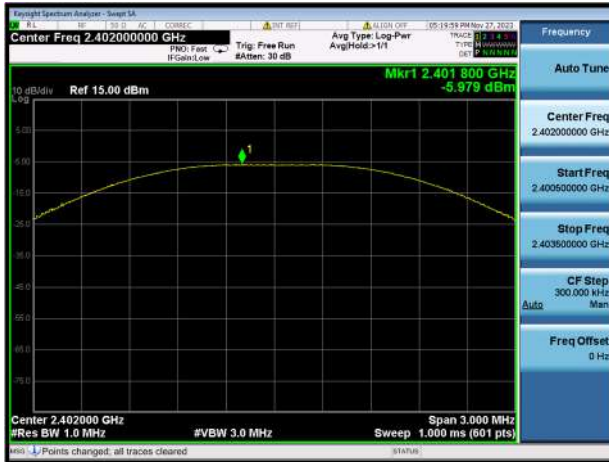
GFSK (BLE 1Mbps) LOW CHANNEL
