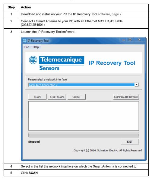
Ethernet Smart Antenna Installing the System
