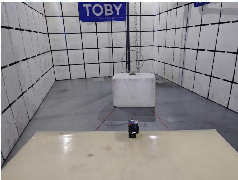
Photo of Setup for Radiated Emission (9KHz-30MHz)
