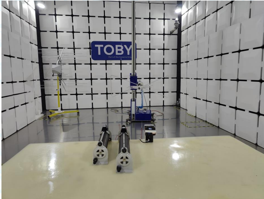
Photo of Setup for Radiated Emission (9KHz-30MHz)
