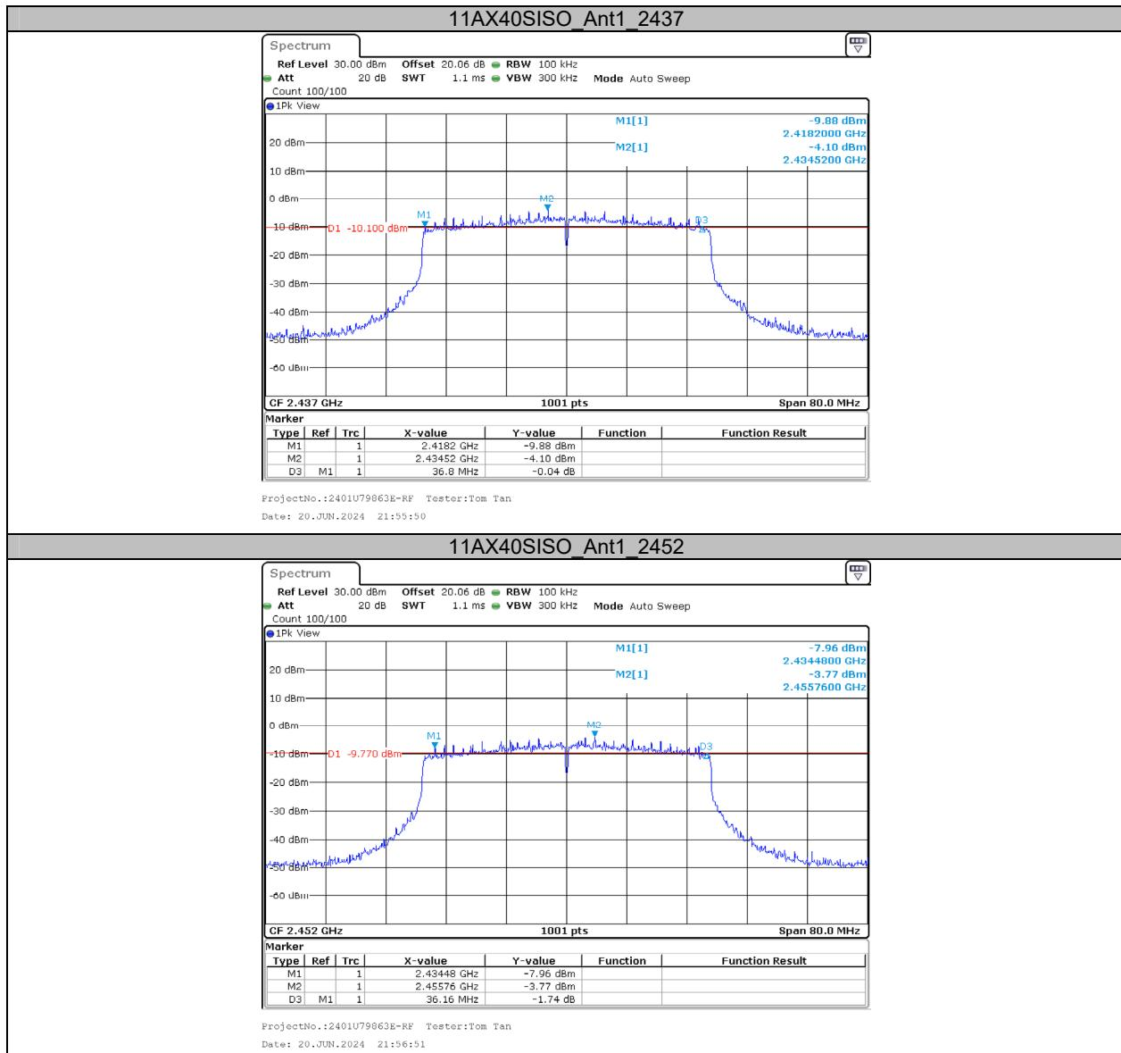
**Appendix B: Occupied Channel Bandwidth****Test Result**
