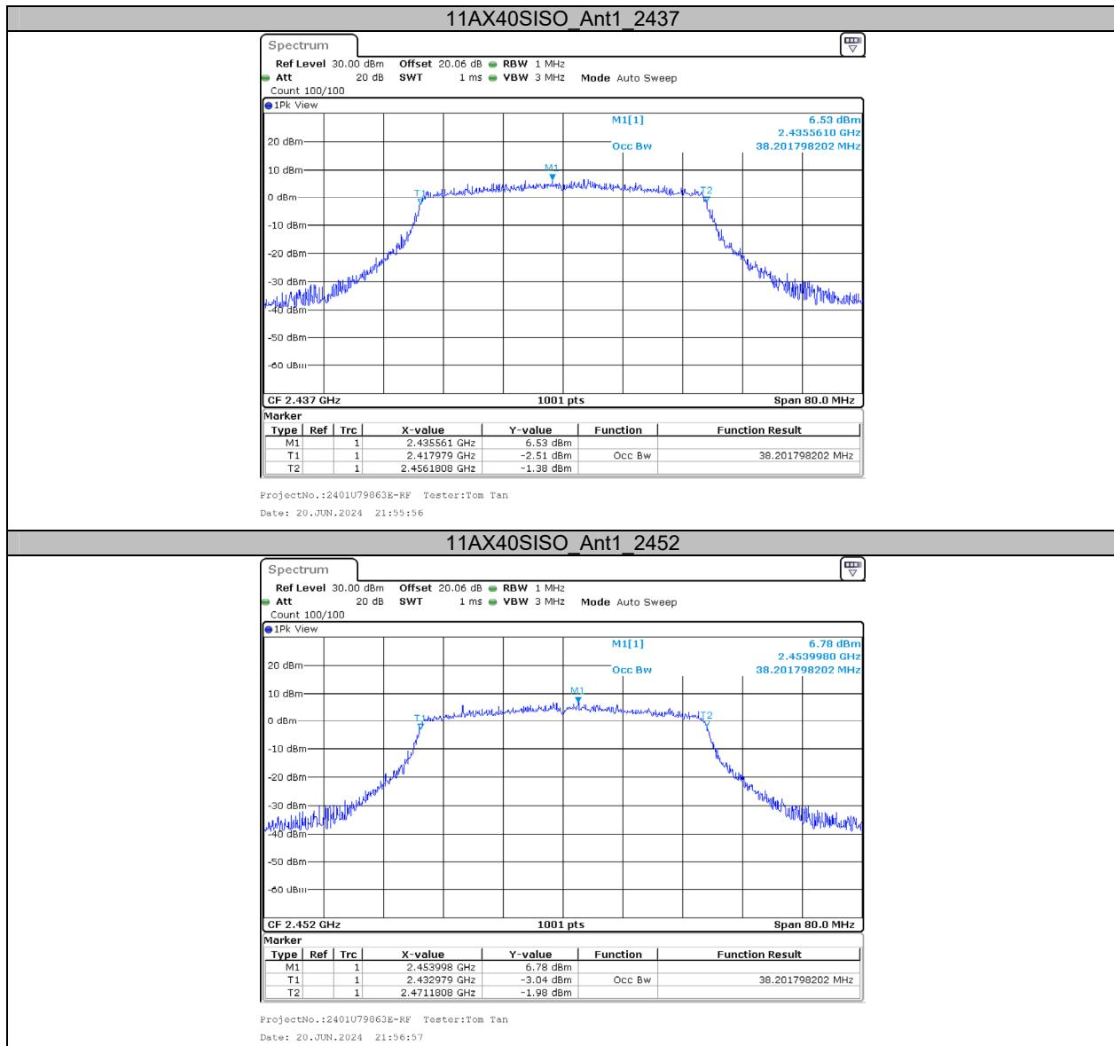
**Appendix C: Maximum Conducted Peak Output Power****Test Result**
