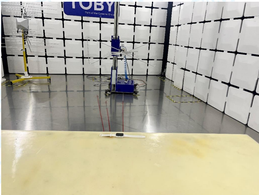
Photo of Setup for Radiated Emission (30MHz~1GHz)
