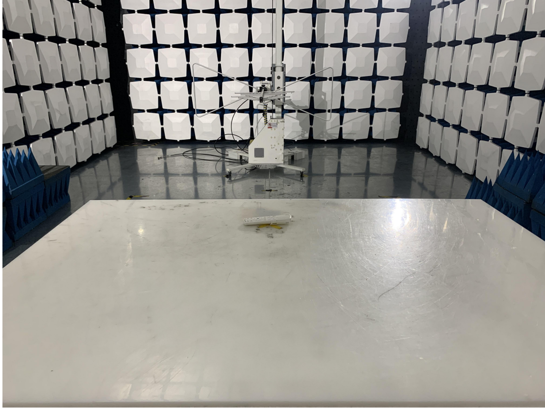
Above 1GHz for radiated emission test setup
