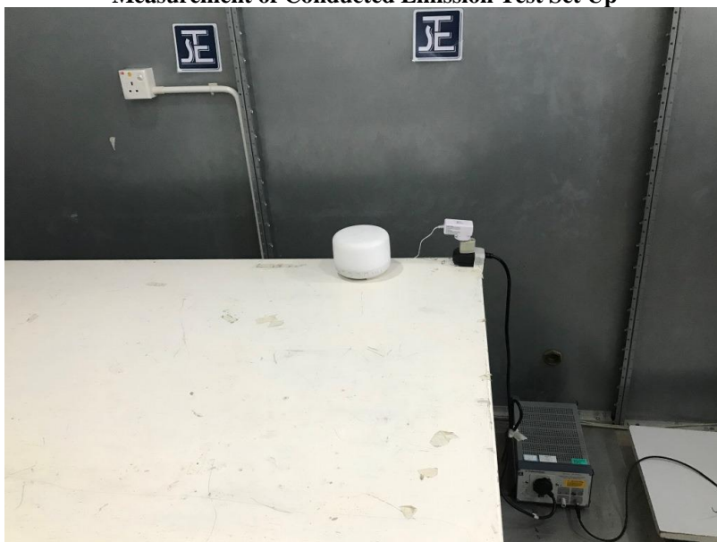
Measurement of Conducted Emission Test Set Up
