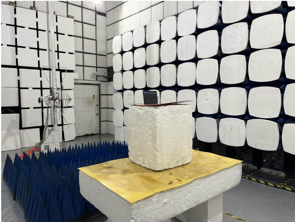
Radiated Emissions Measurement (Below 1GHz)
