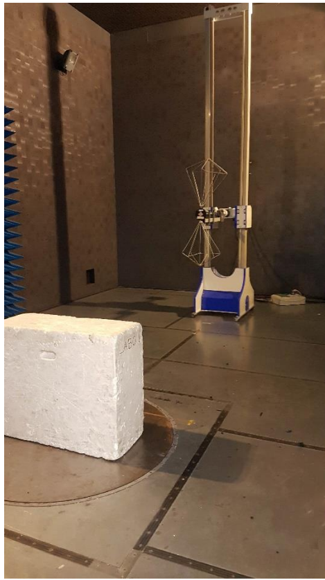
Radiated measurement setup between 200 MHz to 1000 MHz
