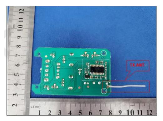
Length: 35mm Antenna Type: Wire Antenna Antenna Gain: 0dBi
